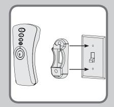
To install the transmitter cradle, remove the two screws holding your switch cover plate. Do not remove the cover plate. Orient the cradle by lining up the two mounting holes with those on the cover plate. Insert and tighten the screws. Do not over tighten.
