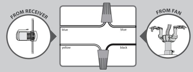
CONNECT WIRES FROM RECEIVER TO FAN - Using the orange wire connectors, connect the blue wire from the receiver to the blue wire (or possibly black with white stripe wire) from the fan. Connect the yellow wire from the receiver to the black wire from the fan.
